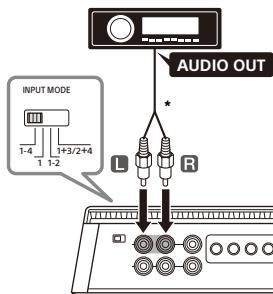
\* Use a speaker wire-to-RCA adaptor (not supplied) for high-level input connection.
