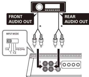
\* Use a speaker wire-to-RCA adaptor (not supplied) for high-level input connection.
