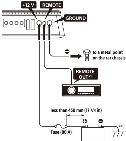
\*1 If you have the factory original or some other car audio unit without a remote output for the amplifier, connect the remote input (REMOTE) terminal to the ACC power supply. In high level input connection, the amplifier can also be activated without a need for REMOTE connection. However, this function is not guaranteed for all car audio units.
