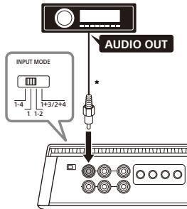
\* Use a speaker wire-to-RCA adaptor (not supplied) for high-level input connection.
