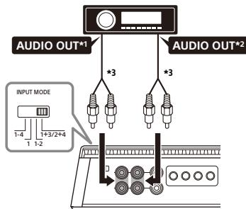
\*1 Filtered signal. Tweeter output or HPF output from the car audio.
